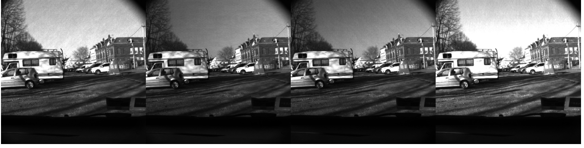
Figure 3.1: Example of a polarimetric image. From left to right, the intensities corresponding to the polarizer rotation angles 0^\circ , 45^\circ , 90^\circ and 135^\circ .
